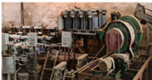
Pilot flotation line with capacity 150 kg/h
